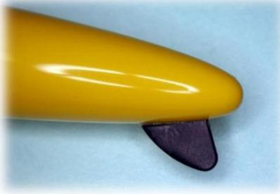
**Figure 11: Shows Landing Skeg Installed**
