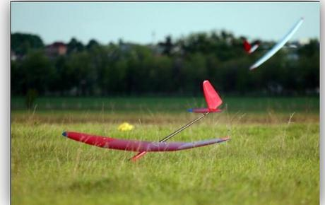
The Supra Pro is the latest version of the Supra - a highly competitive, composite, hollow-molded wing sailplane based on a design by Dr. Mark Drele.
