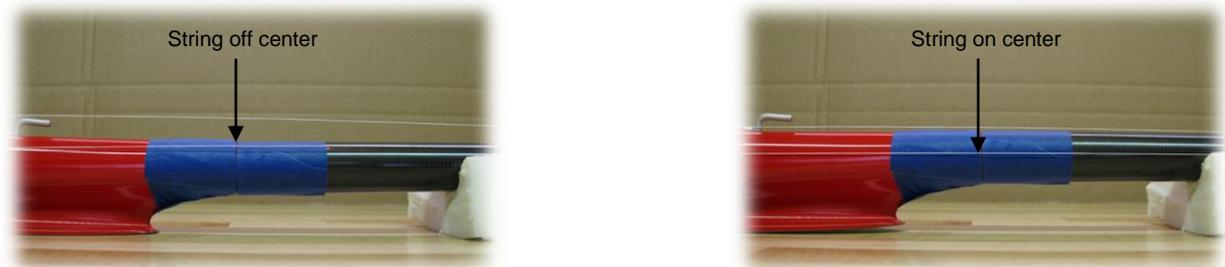
**Figure 7: Shows misalignment on the left and alignment on the right**
