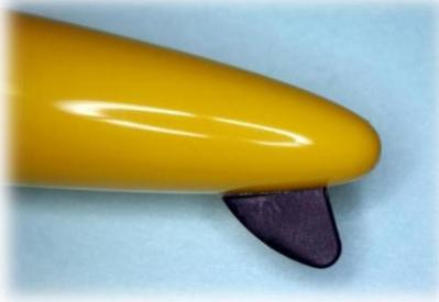
**Figure 11: Shows Landing Skeg Installed**
