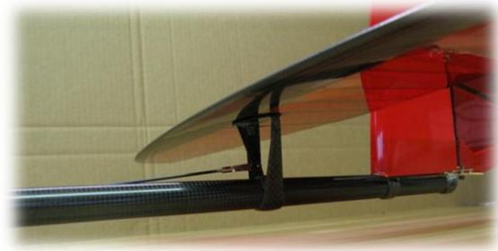
**Figure 16: Shows the Stabilizer and Stabilizer pushrod installed**
