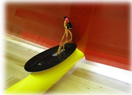
**Figure 22: Connect the Wing wire harness**
