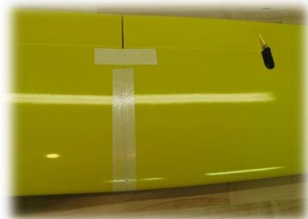
**Figure 26: Wing tip taped to Wing center section**
