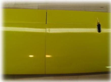
**Figure 25: Wing tip installed on Wing center section**
