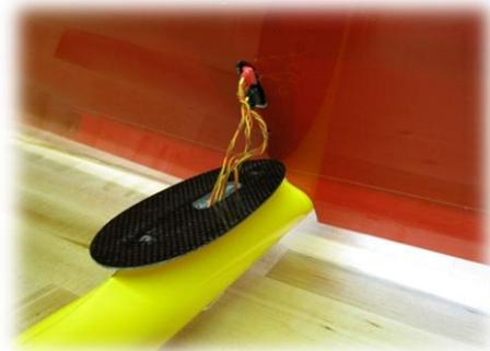
**Figure 22: Connect the Wing wire harness**
