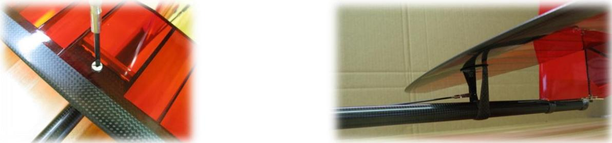
**Figure 16: Shows the Stabilizer and Stabilizer pushrod installed**
