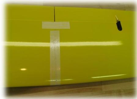
**Figure 26: Wing tip taped to Wing center section**
