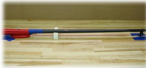
**Figure 5: Shows fuselage and boom epoxied together, and secured to the table**
