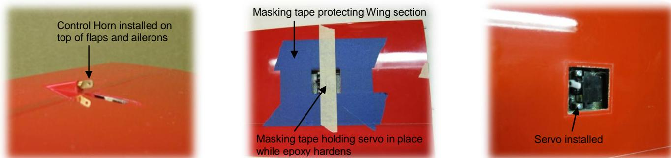
**Figure 18: Shows a control horn installed, shows a servo being installed, and a servo installation completed (Pushrod not shown for clarity)**
