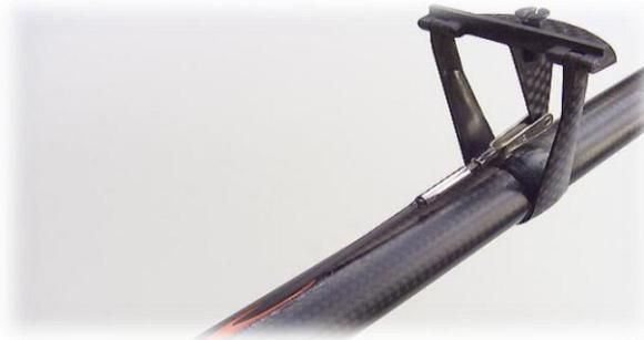
**Figure 12: Stabilizer pushrod clevis installed on v-mount**
